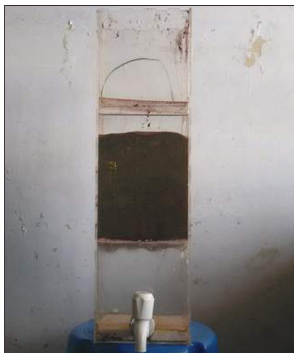
Fig. 4.2.7(b). Uncoated sand filled in material container
