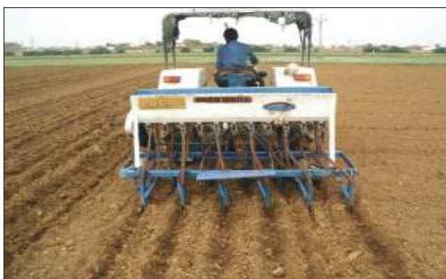
Plate 2.8.3. Sowing of crop by seed cum fertilizer drill and irrigation through long border strip
