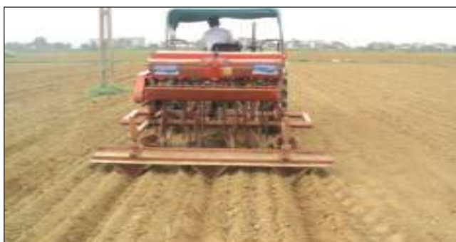
Plate 2.8.4. Sowing of crop by broad bed seed cum fertilizer drill and furrow irrigation
