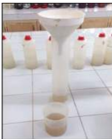
Fig. 3.1.3. Determination of silt in runoff and recharge water
