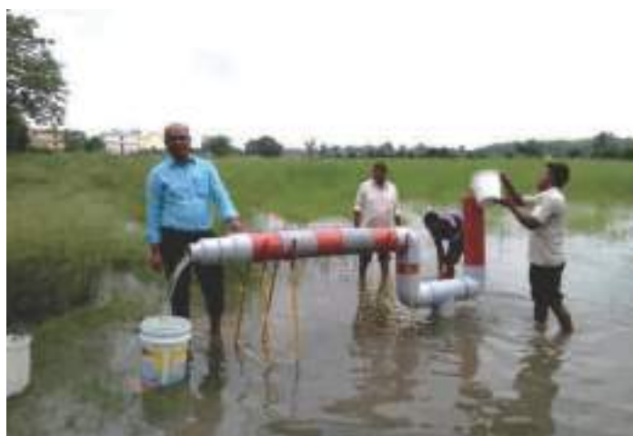
Plate 3.3.1. Filter assembly testing under field condition using runoff water
