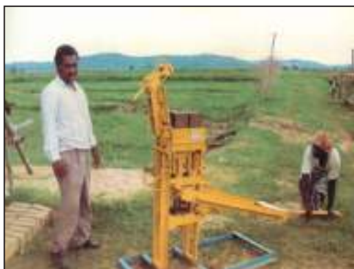
Manual soil block press for making mud blocks and tank with mud block and LDPE film
